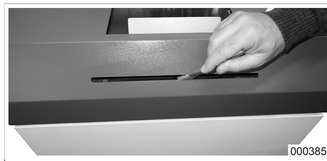
Fig.11 Cleaning the photocells
