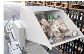
Efficient PET recycling system to reduce the volume of empty PET bottles by up to 90 % and produce compact raw material bales
