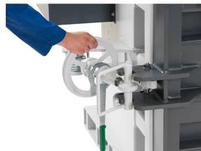
Hand wheel door lock - Easy to handle thanks to counter-rotating thread for quick opening and closing
