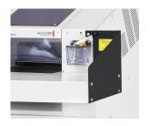
To ensure a consistently high cutting capacity, shredder baler combinations with cross cut have a manual oiler.
