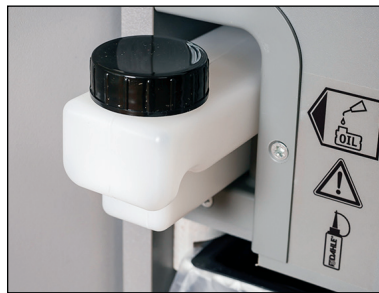
EvenFlow Lubricator evenly oils the cutting cylinders to ensure peak performance.
