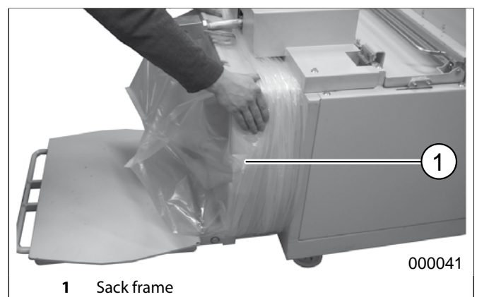
fig. 19 Installing a new plastic sack
